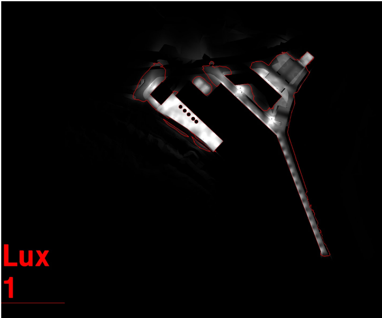
Figure 10 – Greyscale rendering of site with 1 lux horizontal illuminance contour line at ground level to show spill of light outside of boundary, considering the 3D topographic model
